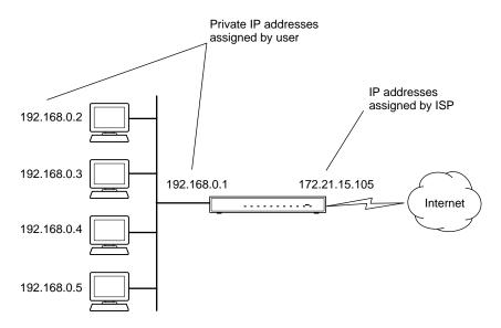
Figure B-3: Single IP Address Operation Using NAT
